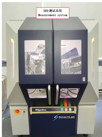
Rigaku SmartLab is a full-featured high-resolution X-ray diffractometer (XRD). The equipment accepts powder, bulk, films samples, and measurements can be performed with the new Rigaku SmartLab Studio II software suite, which is an integrated software platform incorporating all functions from measurement to analysis.
